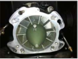
To make sure that you have connected the top right screw properly, gently wiggle the elbow back and forth the ensure that you have tightened the screw correctly so that the elbow doesn't slide around.
